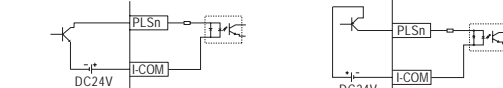
*4 The Input Common (I-COM) shown here is connected to a Sink Output type. (The dotted line shows the connection with a Source Output type.)
